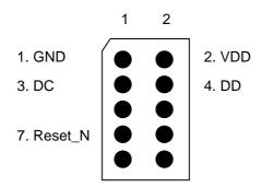
Figure 4: Recommended debug connector layout (Top view)
